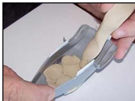
Fill the inside of the Model with Klean Klay, ensuring all openings are covered.
