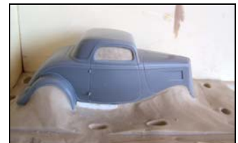
Embed the Model in clay on mould box base. Add holes for registration keys.
