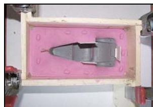
Rebuild mould box. Apply release agent.
