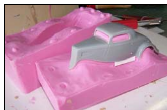
Turn the silicone block over and carefully remove clay. DO NOT remove the model from the mould
