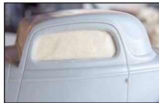
On outside, clean and smooth edges of all openings.
